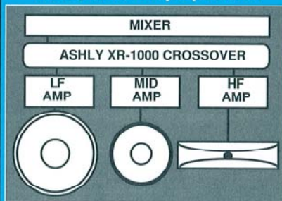
Typical Hookup Of XR-1000 in Mono, Three-Way Operation
