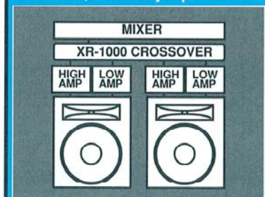
Typical Hookup Of XR-1000 in Stereo, Two-Way Operation
