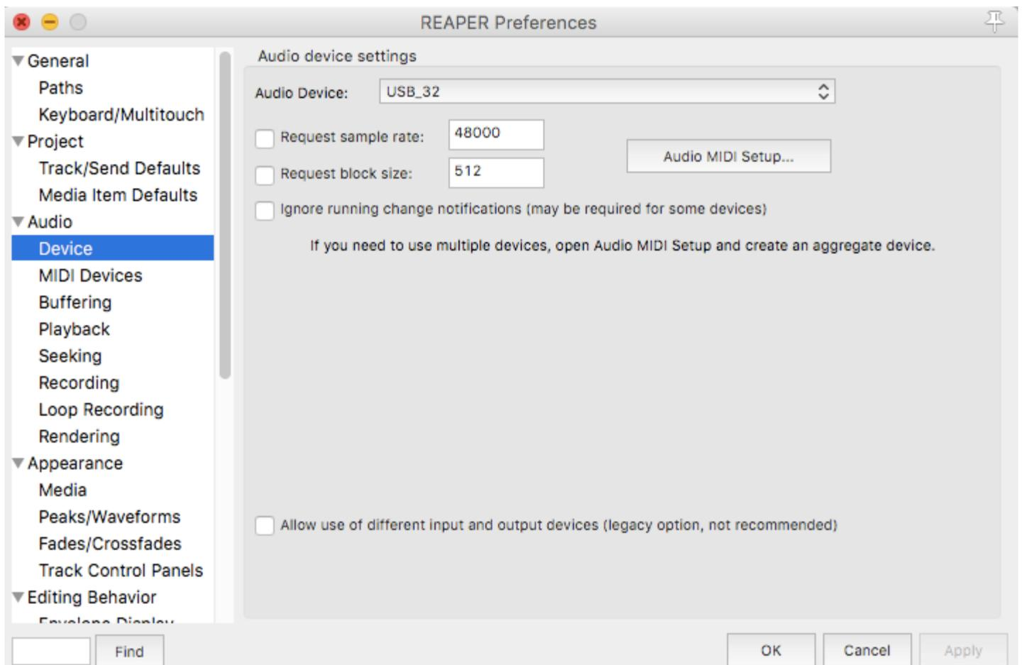
**1.2 - For Windows® PCs's**, USB driver software specifically for the digiMIX24 must first be installed. Obtain the Ashly digiMIX USB-32 USB driver software from Ashly web site and extract the files from the download. With the computer not yet connected to the digiMIX24, install the driver software as described below. The installation windows are slightly different for the different versions of the Windows operating system, but the basic procedure is the same.
