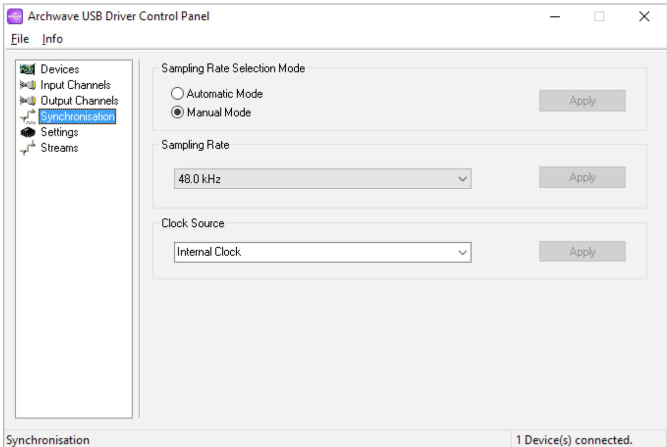
**The digiMIX24 only operates at a 48 kHz sample rate, and the USB-32 driver software must be selected for 48.0 kHz for the USB-32 option to work.**
