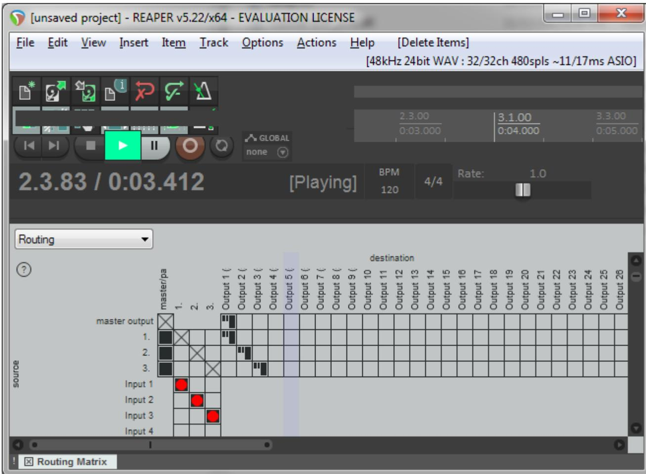
In your multichannel recording software, you may need to assign the recorded tracks to output channels. Shown above is an example of routing, or assigning, tracks to outputs. Within the digiMIX24, channel mapping is fixed, but you can view it by pressing the mixer touchscreen <Digital In> button, then <Channel Mapping>.
