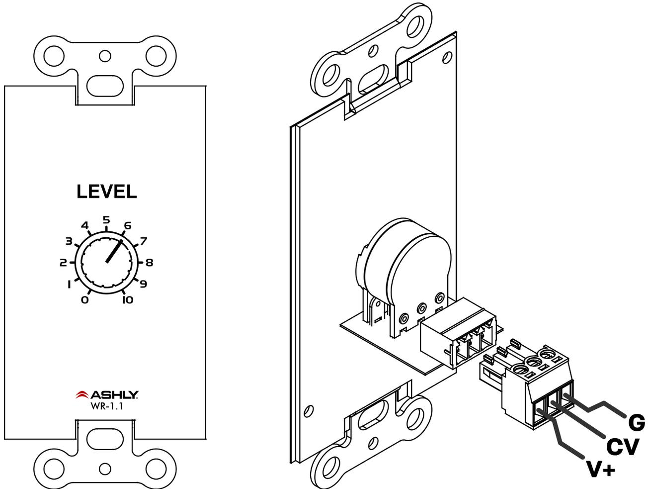
The WR-1.1 is a remote level control for all Ashly products with DC level control inputs on Euroblock connectors. It is designed to fit into a single North American electrical wall box. A decorative cover can be purchased separately at an electrical hardware supplier.
