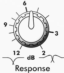
Dial calibrations refer to the amount of attenuation effected by the filter at the crossover frequency, i.e., a setting of 3dB means that the filter's hi-pass and low-pass outputs are each "rolled off 3dB at the crossover point". This describes Butterworth filter response, or a gentle 3dB peak at the crossover point when the two filter output signals overlap.
