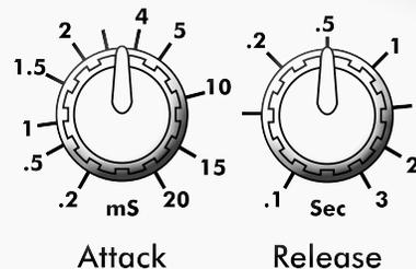
A unique feature of CLX-52 is the incorporation of a *Double Release Time Constant*. When a conventional compressor/limiter is adjusted for slow release times, transients such as mic “pops” may cause a severe reduction in gain followed by a slow fade up, making the action of the limiter very obvious.
