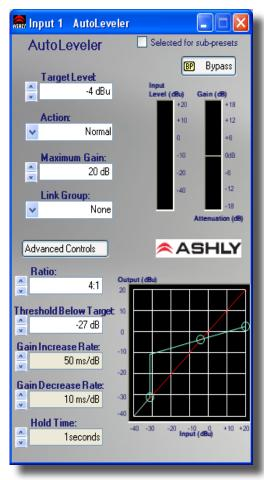
**Maximum Gain** - This is the total amount of gain the auto leveler may apply before it stops affecting the signal. Maximum Gain controls the Threshold Below Target using the following formula:
