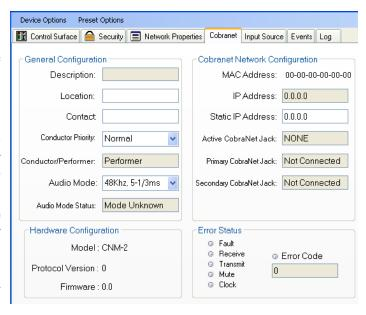
Audio Mode Status: The current Audio Mode of the Unit. If a mode is not supported this status may not equal the selected mode.
