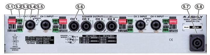
**5.1 Channel Configuration DIP Switch** - The DIP switches configure each channel's 80Hz 2nd Order Hipass Filter, Output Clip Limiter, Amplifier Gain, and Output Mode. In the example to the right, the DIP switch is set as follows: 6: 80Hz High Pass Filter is Off; 5: Clip Limiter is On; **4&3**: Gain is <u>1.4V</u>; **2&1**: Output Mode is <u>Low Z</u>.
