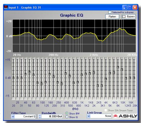
**Bandwidth** - This sets the Bandwidth of the filters, from 1/4 octave to 1/2 octave (before Proportional Adjustment). The default bandwidth is 1/3 octave.
