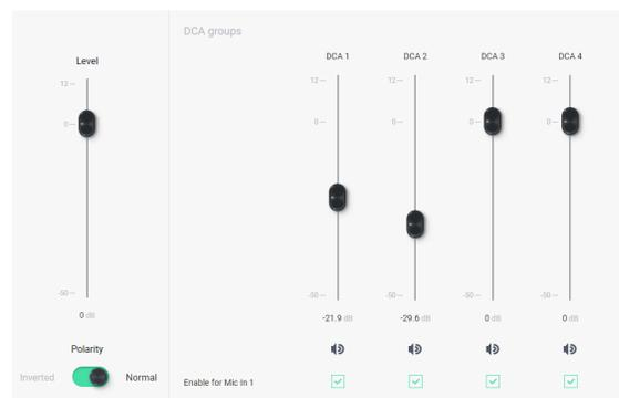
A DCA gain block can be placed on any channel in order to make that channel available for DCA groups 1-4. Each DCA block must be turned ON to be active. Each DCA block must also be enabled for its targeted DCA group.
