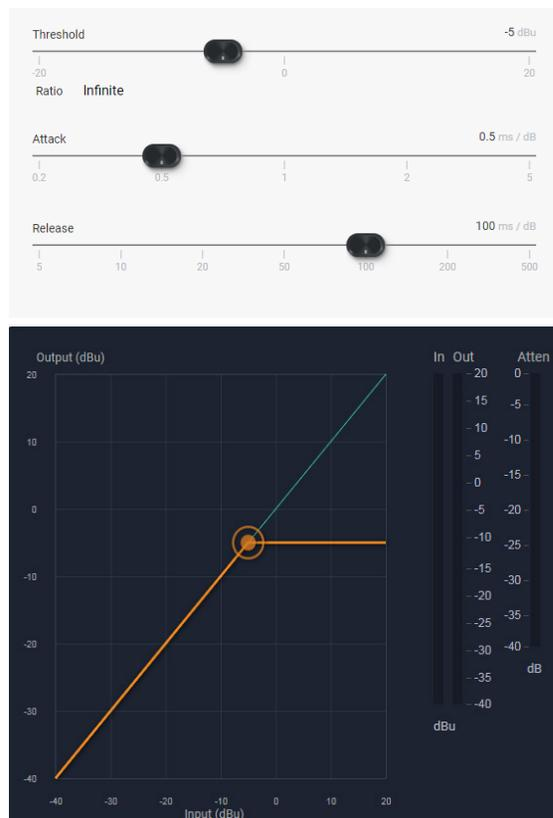
The brick wall limiter is a compressor with a fixed infinite ratio. Use this limiter to prevent signal from exceeding a designated peak level. The limiter has threshold, attack time and release time adjustments.
