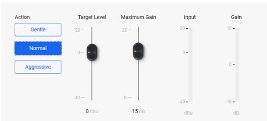
**Target Level** - This is the desired continuous output level of the signal.
