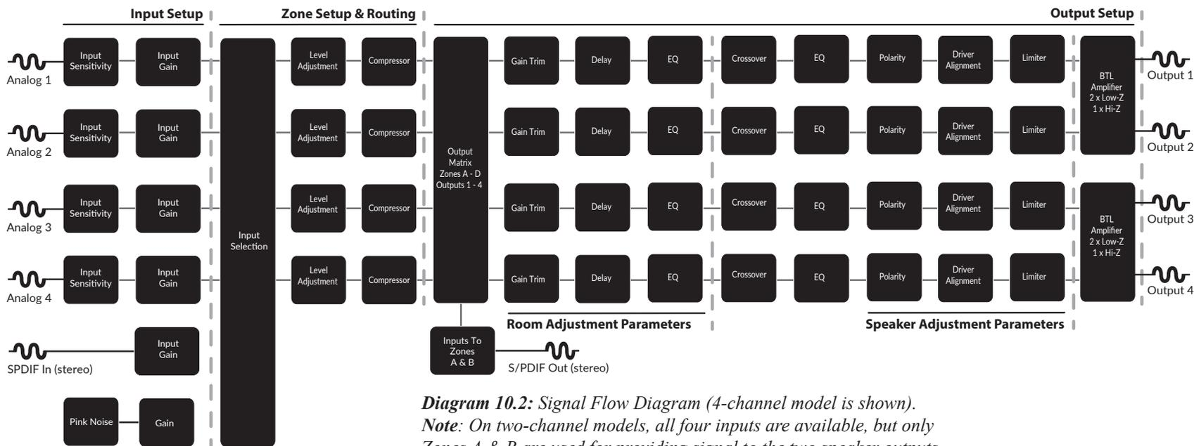
**Diagram 10.2:** Signal Flow Diagram (4-channel model is shown).
