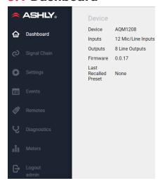
The AQM1208 dashboard screen is the home page after launching the software. All configuration menus are found here, as well as device & firmware information, plus the last recalled preset. Menus include the following:
