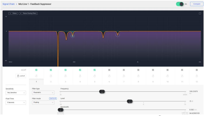
The **Sensitivity** control has five levels. This adjusts how sensitive the FBS algorithm is to detecting feedback and inserting filters. For example, a setting of <Very Sensitive> means the algorithm will aggressively look for anything that could be feedback and hence, may insert filters on sustained musical tones.
