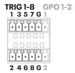
Eight programmable trigger inputs are available for contact closure events. The triggered event occurs when the trigger input pin is connected to its ground using a contact closure switch.
