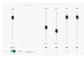
A DCA gain block can be placed on any channel to make that channel available for control within DCA groups 1-4.
