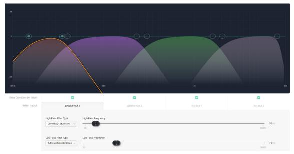
Crossover blocks can be placed on any output channel. A high-pass and low-pass filter type and frequency get applied to each crossover block to band-limit the signal for that output.
