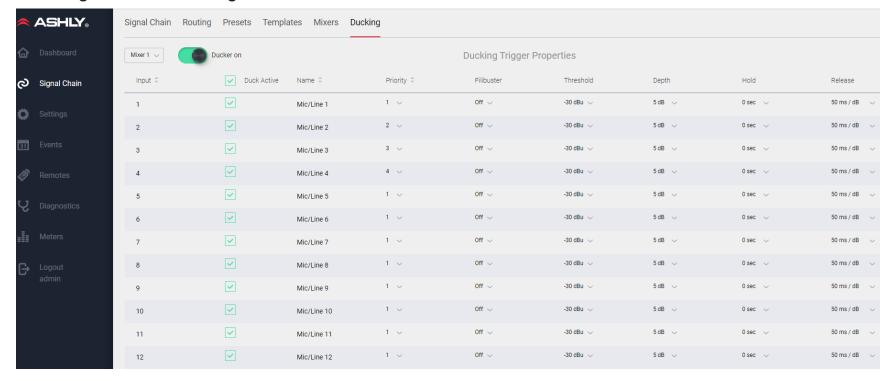
This dedicated ducking setup screen is used for easy editing and at-a-glance visibility of all ducking trigger properties.
