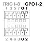
Two GPO (general purpose output) pins are available for driving external device logic inputs to effect a lighting change, motorized curtain, projector screen, etc. GPO logic status can be recalled as part of a preset, sub-preset, or changed using a scheduled or triggered event.
