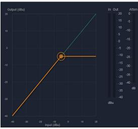
The brick wall limiter is a compressor with a fixed infinite ratio. Use this limiter to prevent signal from exceeding a designated peak level. The limiter has threshold, attack time and release time adjustments.
