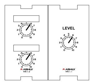
The WR-1 and WR-1.1 are remote level controllers used for DC level control inputs. The WR-1 (dual potentiometer) and WR-1.1 (single potentiometer) mount to a standard North America electrical wall box. The remote is wired to the AQM1208 Euroblock VCA pins V+, 1, 2, or 3, and ground, then associated in software with a VCA Gain block placed anywhere in the signal chain.
