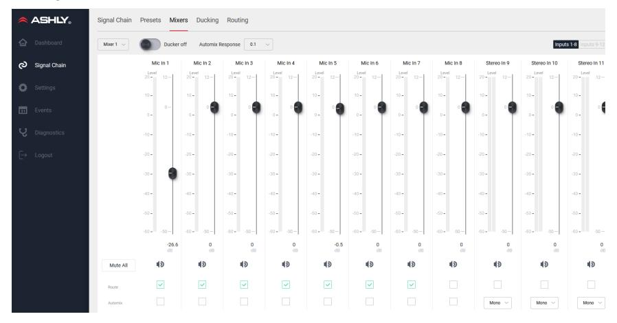
All input channels can be independently routed and mixed to all eight mixers. The eight output channels can then use any one of the eight mixers as their source. If desired, the same mixer can be used on multiple output channels.
