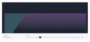
A high-pass filter (HPF) is a single ended filter without a level control, passing only signal above the selected corner frequency. Filter types include Bessel, Butterworth, Linkwitz, and Linkwitz Notch, offering a variety of filter slope values.
