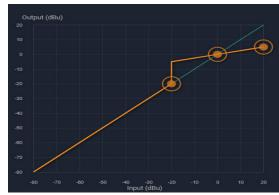
The auto leveler is a dynamics processor used to automatically boost or cut a signal to maintain a user-defined target level.
