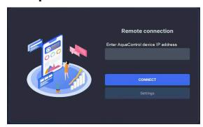
After wiring to the network and booting the AquaTouch7, the above Remote Connection screen appears.
