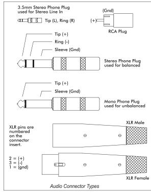
Two-conductor (twisted pair) shielded cable is best for all XLR type connections. Belden No. 8412, or its equivalent, is an excellent cable due to its heavy construction. This type of cable should be used for all portable applications. Snake cables containing multiple shielded pairs must be handled very carefully because the leads tend to be fragile, and a broken conductor is difficult to repair.
