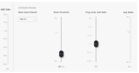
Ambient noise compensation (ANC) is an automatic output level control that uses a microphone monitoring a zone's ambient background noise to adjust overall output level for that zone, automatically maintaining intelligibility above the ambient noise.
