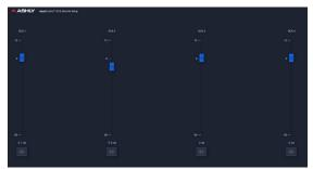
DCA groups are used to globally adjust the relative levels of all channels assigned to that group. In the DSP signal chain, a DCA block must first be placed on every channel you wish to assign to a DCA group, then enabled and adjusted for each DCA group as desired. A remote Operator role is then created granting permission to use a DCA Remote on a tablet or mobile device.
