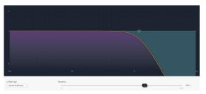
A low-pass filter (LPF) is a single ended filter without a level control, passing only signal below the selected corner frequency. Filter types include Bessel, Butterworth, Linkwitz, and Linkwitz Notch, offering a variety of filter slope values.
