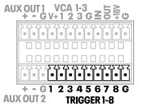
Eight programmable trigger inputs are available for use with contact closure switches.
