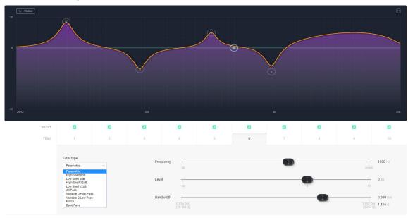
The PEQ parametric equalizer offers a variety of useful filter types for adjusting signal response with greater precision. A master on/off button enables/disables the PEQ block.
