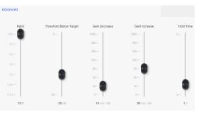
**Threshold Below Target** - Determines the relative input signal level above which the autoleveler increases gain, below which no action is taken.
