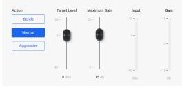
**Target Level** - This is the desired continuous output level of the signal.
