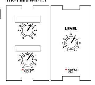
The WR-1 and WR-1.1 are remote level controllers used for DC level control inputs. The WR-1 (dual potentiometer) and WR-1.1 (single potentiometer) mount to a standard North America electrical wall box. The remote is wired
