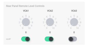
Three back-panel VCA (voltage controlled amplifier) input pins are used to remotely control the level of assigned inputs or outputs using a simple potentiometer circuit.
