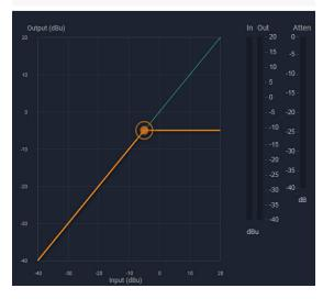
The brick wall limiter is a compressor with a fixed infinite ratio. Use this limiter to prevent signal from exceeding a designated peak level. The limiter has threshold, attack time and release time adjustments.
