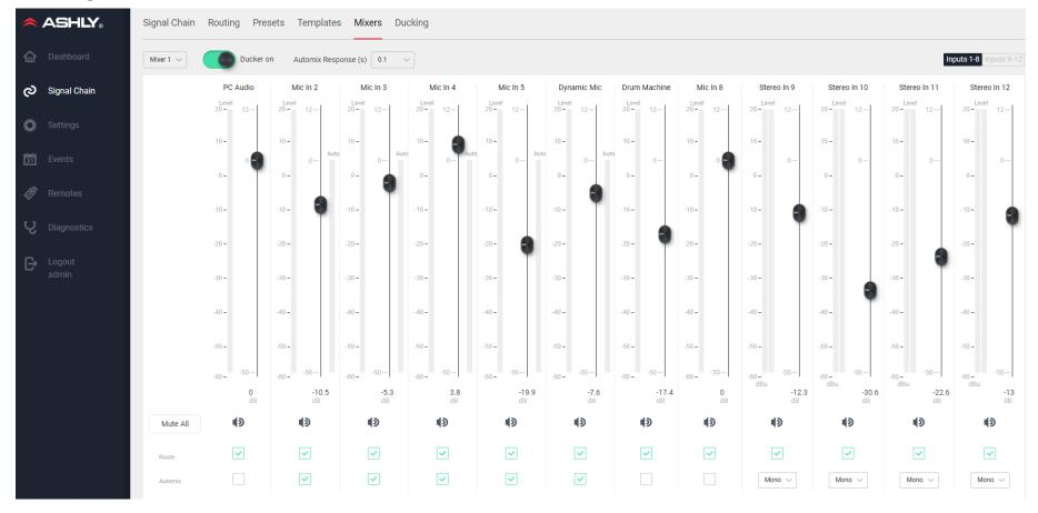
Four independent mixers can be assigned to the two amplifier outputs or two aux outputs. Each mixer offers independent input channel level control, routing, mixer mute, ducking enable, automix assignment, and automix response time. Stereo input channels 9-12 can be set for left input only, right input only, or summed mono.
