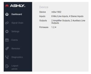
The dashboard is the first page you see after logging in with your browser. The dashboard shows the Ashly device, number of inputs and outputs, and installed firmware revision.
