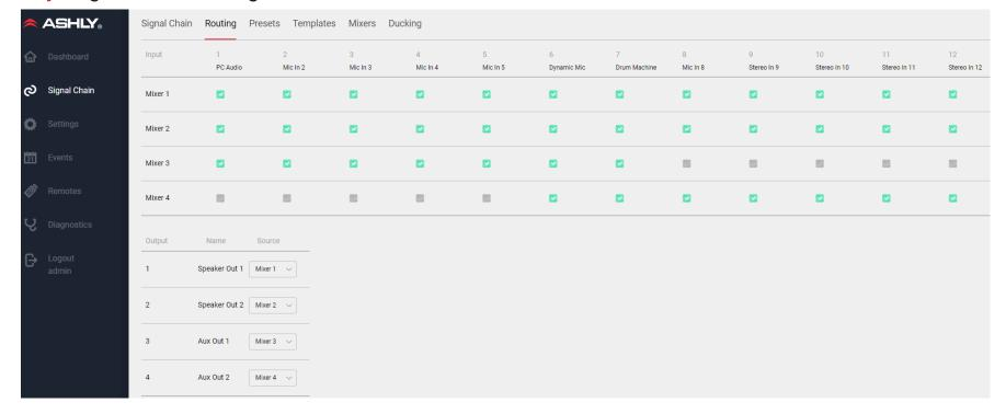
The signal chain routing page provides fast setup and review of all 12 input channel routings to all four mixers.
