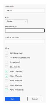
Typical use of the Operator role might be for deploying a Remote Mixer, Remote DCA, remote Virtual WR5, or AquaTouch7 to a secure but limited access user, or for granting the operator signal chain or preset recall access.
