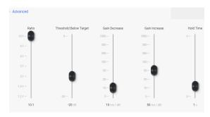
Threshold Below Target - Determines the relative input signal level above which the autoleveler increases gain, below which no action is taken.
