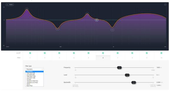
The PEQ parametric equalizer offers a variety of useful filter types for adjusting signal response with greater precision. A master on/off button enables/disables the PEQ block.
