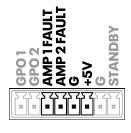
into protect mode, the amp fault output pin for that channel goes logic low.
