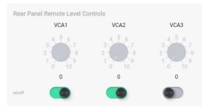
Three back-panel VCA (voltage controlled amplifier) input pins are used to remotely control the level of assigned inputs or outputs using a simple potentiometer circuit.
