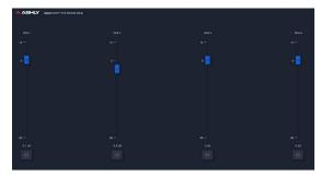
DCA groups are used to globally adjust the relative levels of all channels assigned to that group. In the DSP signal chain, a <u>DCA block</u> must first be placed on every channel you wish to assign to a DCA group, then enabled and adjusted for each DCA group as desired. A remote Operator role is then created granting permission to use a DCA Remote on a tablet or mobile device.
