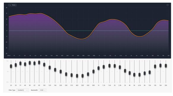
The graphic equalizer offers 31 standard ISO center frequency controls with constant Q or proportional Q filters, as well as adjustable filter bandwidth.
