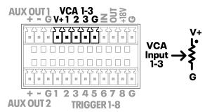
Remote DC level control is available on these three VCA (voltage controlled amplifier) inputs. A VCA Gain block must first be placed in an input or output signal chain, then assigned to a VCA input. Multiple VCA gain blocks can be assigned to the same VCA input pin.
