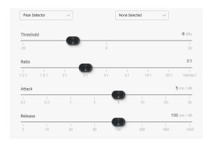
**Threshold** - The signal level at which the compressor begins to apply gain reduction to the signal. Threshold range is -20dBu to +20dBu.
