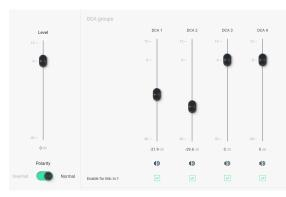
A DCA gain block can be placed on any channel in order to make that channel available for DCA groups 1-4. Each DCA block must be turned ON to be active. Each DCA block must also be enabled for its targeted DCA group.
