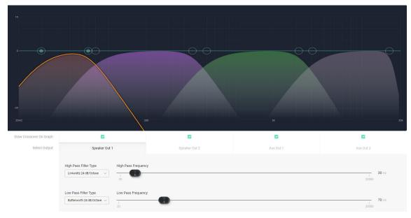
Crossover blocks can be placed on both speaker and Aux output channels. A high-pass and low-pass filter type and frequency get applied to each crossover block to band-limit the signal for that output.
