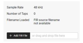
Plugging in a FIR filter DSP block then clicking on it will prompt the user for a \*.fir, \*.txt, or \*.csv text file, which is then loaded and applied to the output DSP. The two file types have identical coefficient code, however the \*.fir file may add comments (designated by a semi-colon) or a key=value pair definition such as sample rate. Both file types will work in AquaControl.
