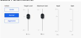
**Target Level** - This is the desired continuous output level of the signal.
